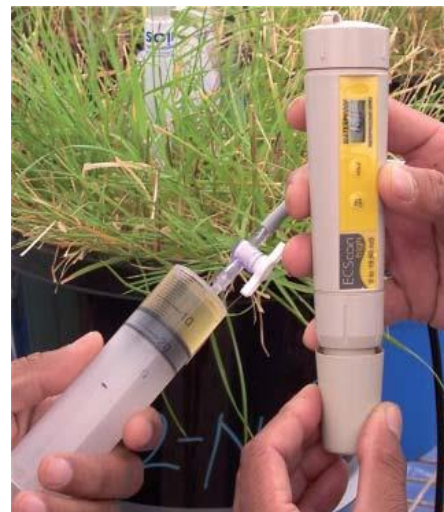
Figure 6 Extracting sample and reading the EC meter
